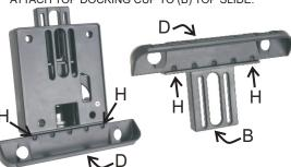
3. USING (E) SCREWS AND (F) NUTS, ATTACH TOP SLIDE TO INTERNAL TAB-LOCK  $^{\rm TM}$  SLIDE AS SHOWN. DO NOT FULLY TIGHTEN. (SLIDES MUST REMAIN LOOSE)
