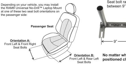
Seat bolt range must have a **center to center** distance between 9" and 19".
