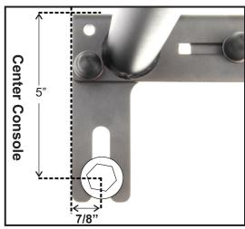
If you are using Orientation B from Step 1, the distance between the seat bolts and center console must be at least 5".
