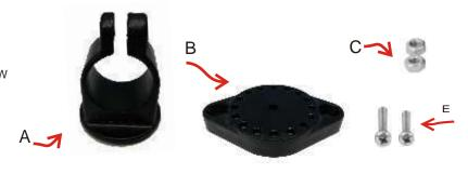
The RAM Rail Mount consists of a locking tooth system with a standard RAM diamond plate end. The mount will fit a rail diameter from 1.0" to 1.1". You can place a rubber lining or electrical tape (not included) between the tube and the mount for a tube with a diameter less than 1". This will help the base grab the rail.
